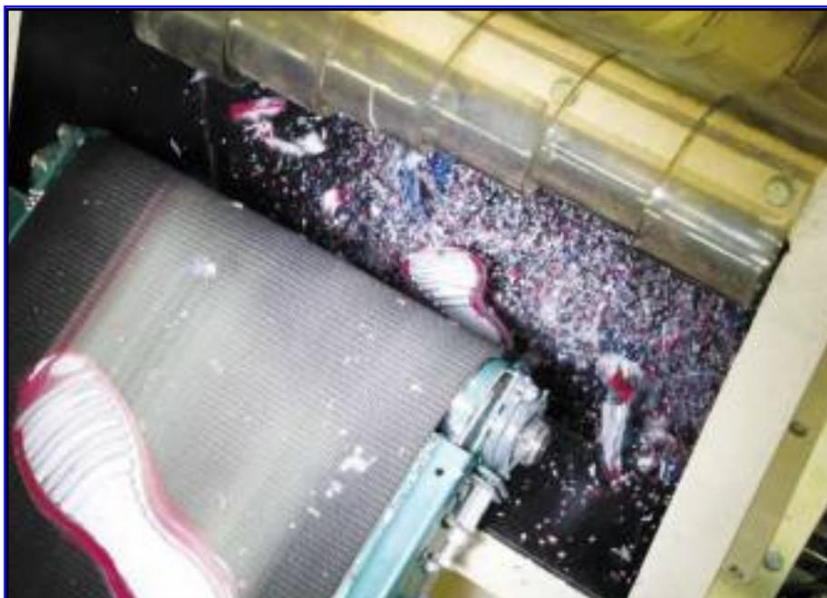
Grinding up old sneakers at Nike's sneaker recycling plant.
